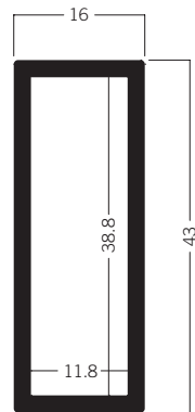
Z 100* Beam extrusion 43 mm 3.14 kg
